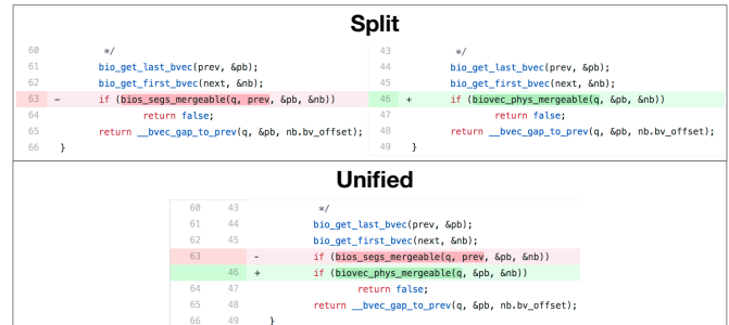
Figure 1: Unified and Split Representations: Source code change done in the function bio_will_gap in the GitHub Linux project.
